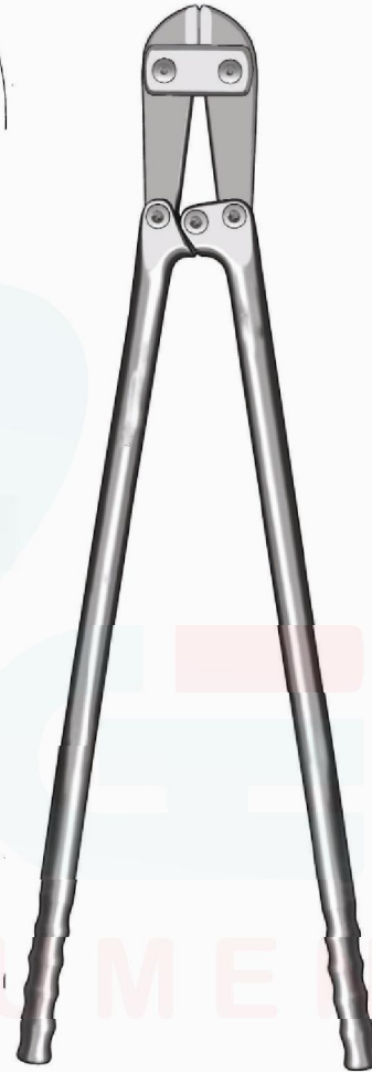
PIN CUTTER (LARGE) 22-528-00 22" (559mm) side cutting cuts up to ¼" (6.3mm)
