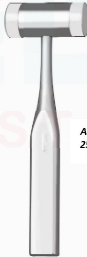
MALLET lightweight 23-240-09 7 ½" (191mm) with two replaceable nylon caps anodized aluminum handle weight: 7 oz. (200 grams) head weight: 4 oz. (120 grams) head diameter: 25mm
