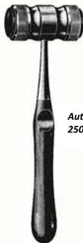
MEAD Mallet E33693-32 7 1/2" (191mm) with replaceable nylon caps weight: 11 oz. (315 grams) head weight: 6 oz. (170 grams) head diameter: 20mm
